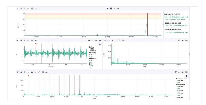
The report indicated there was looseness in the bearing due to improper clearance or fit. The mill personnel immediately made plans to remove the top of the pillow block bearing to examine and verify the findings on September 22<sup>nd</sup>. Our partner RE&E was also present to assist. Pictures of the bearings housing and outer race are shown below. The outer race as well as the bearing housing showed clear signs of rotation, verifying exactly what the report predicted.
